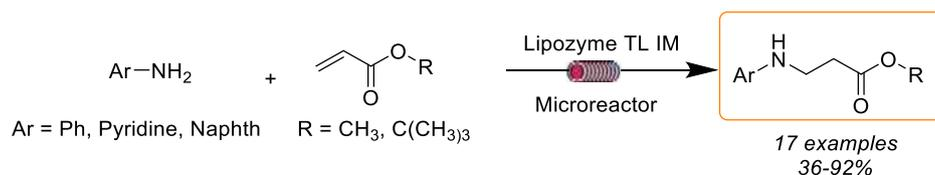
**Scheme 1.** Synthesis of  $\beta$ -amino acid esters by enzymatic Michael reaction of aromatic amines in continuous-flow microreactors.
