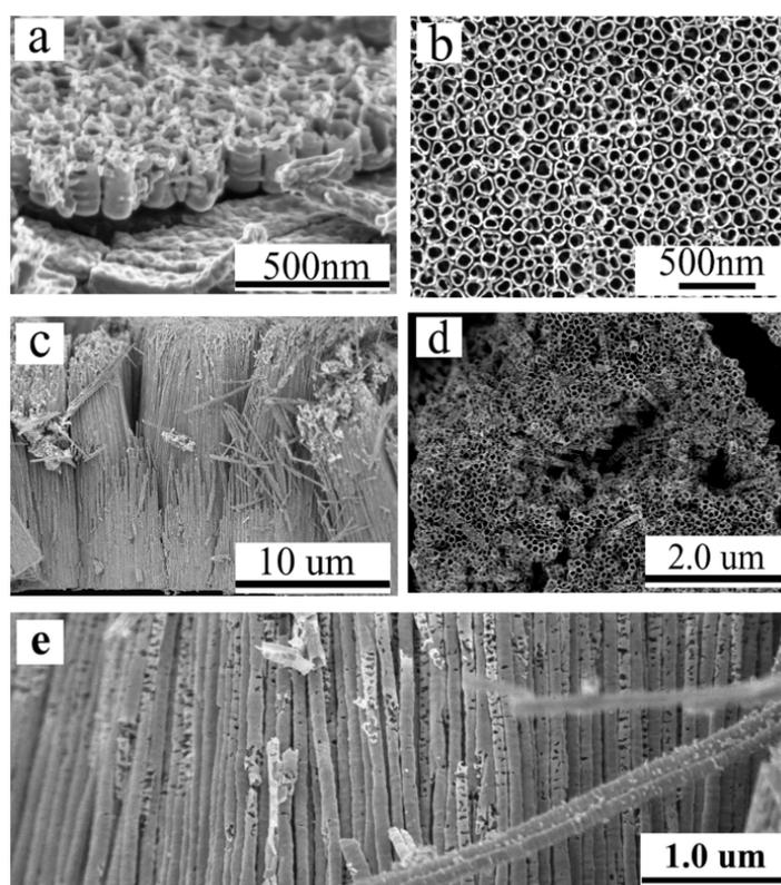
**Figure 9.** Cross-sectional and top-view images of TiO<sub>2</sub> nanotube arrays prepared by anodizing Ti foil at 20 V in 0.5 wt.% HF (Hydrofluoric Acid) aqueous solution for 20 min (a,b) and in formamide-based electrolyte for 6 h (c–e). Reprinted from [16], Copyright 2020, American Chemical Society.
