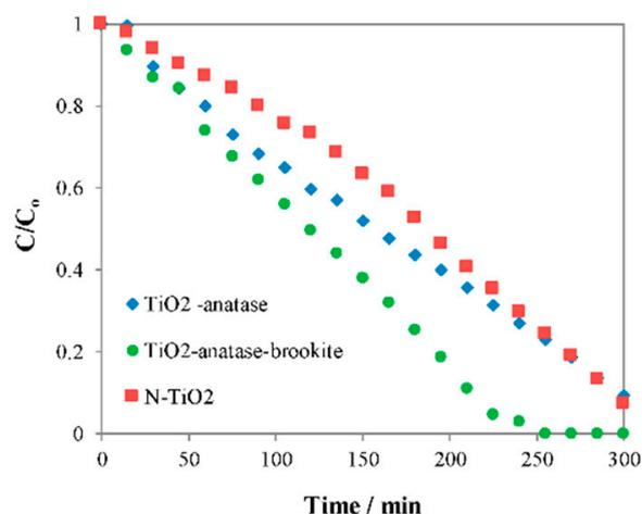
**Figure 6.** Photocatalytic decomposition of acetaldehyde in the circulated flow reactor under UV irradiation on TiO<sub>2</sub> samples prepared by a sol-gel method, the initial concentration of acetaldehyde was around 1800 ppm [35].
