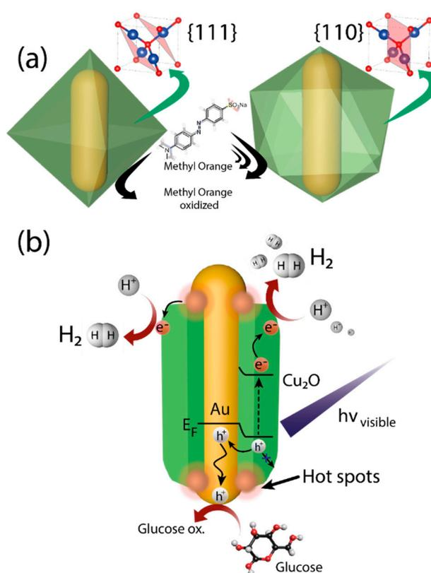
**Figure 7.** (a) Face dependent selectivity of Au@Cu<sub>2</sub>O photoredox catalysis in MO degradation (adapted from [107]) (b) Selective Cu<sub>2</sub>O deposition for partially/completely coated AuNR (adapted from [32]).
