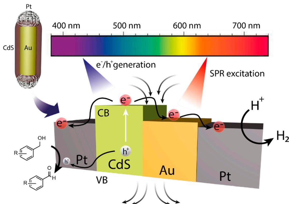
**Figure 10.** Schematic representation of the energy band multichannel in bimetallic@CdS heterostructures (adapted from [136]); semiconductor charge separation under visible light irradiation and its further electron migration through AuNRs to enhance tipped Pt reservoir; Induced both the resonance energy transfer (RET) and hot electron transfer processes and synergistically boosted the photocatalytic reaction (adapted from [136]).
