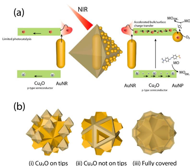
**Figure 8.** (a) Schematic mechanism for methyl orange (MO) photodegradation comparing the binary (left) from the ternary core-shell configuration (right) containing a plasmonic AuNR core, an octahedral  $Cu_2O$  shell and an additional layer of small AuNPs for the ternary alternative (adapted from [113]); (b) Selective  $Cu_2O$  deposition on AuNSs (adapted from [60]).
