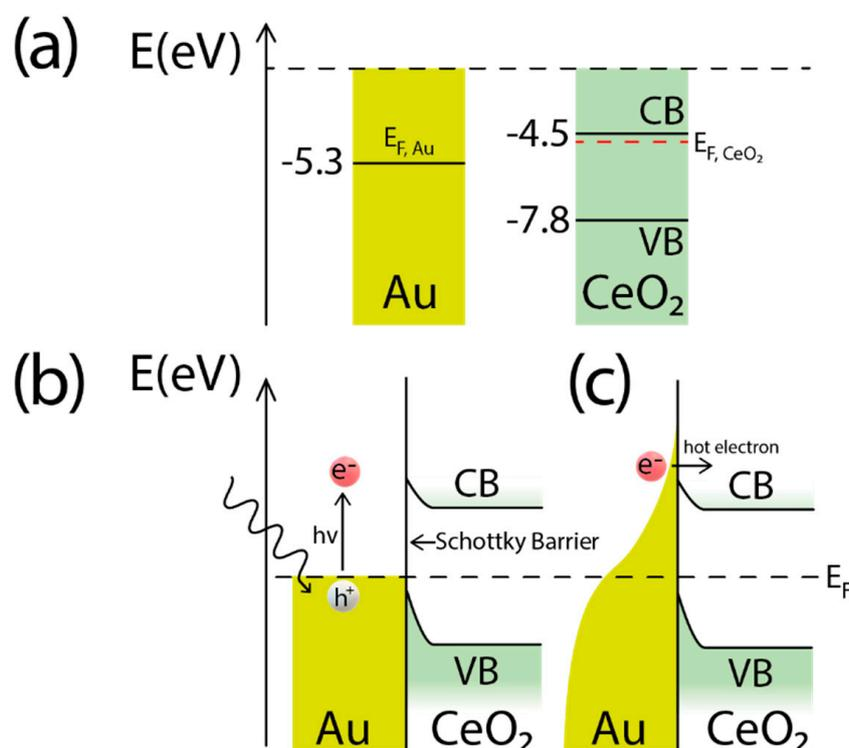
**Figure 4.** Energy band structure of Au-CeO<sub>2</sub> photocatalysts. (a) Energy band levels of Au and CeO<sub>2</sub> respectively; CeO<sub>2</sub> possess a relatively large band gap, needing from UV light to photo-generate charge carriers; (b) energy band distribution upon the gold plasmon excitation to (c) inject hot electrons into the conduction band of CeO<sub>2</sub>.
