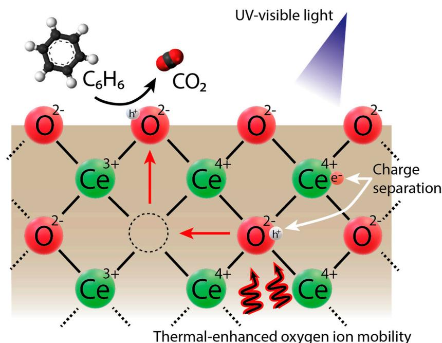
**Figure 6.** Schematic CeO<sub>2</sub> structure remarking the presence of OV and h<sup>+</sup>/e<sup>-</sup> separation. Plasmon-photothermal induced local heating in CeO<sub>2</sub> structure also enhances the oxygen ion mobility, facilitating the migration of O<sup>2-</sup>(h<sup>+</sup>) species to the catalyst surface and, thus, enhancing the reaction (adapted from [89]).
