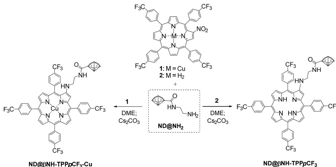
**Scheme 2.** Preparation of porphyrin-functionalized nanodiamonds (ND@βNH-TPPpCF<sub>3</sub>-Cu(II) and ND@βNH-TPPpCF<sub>3</sub>).
