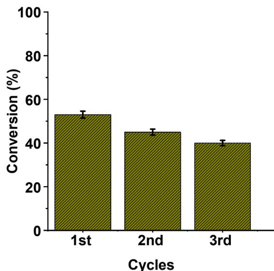
**Figure 5.** Recycling experiments of ND@ $\beta$ NH-TPP $p$ CF<sub>3</sub>-Cu(II) in the oxidation of cyclohexene. Data represent the mean  $\pm$  standard error (n = 3).
