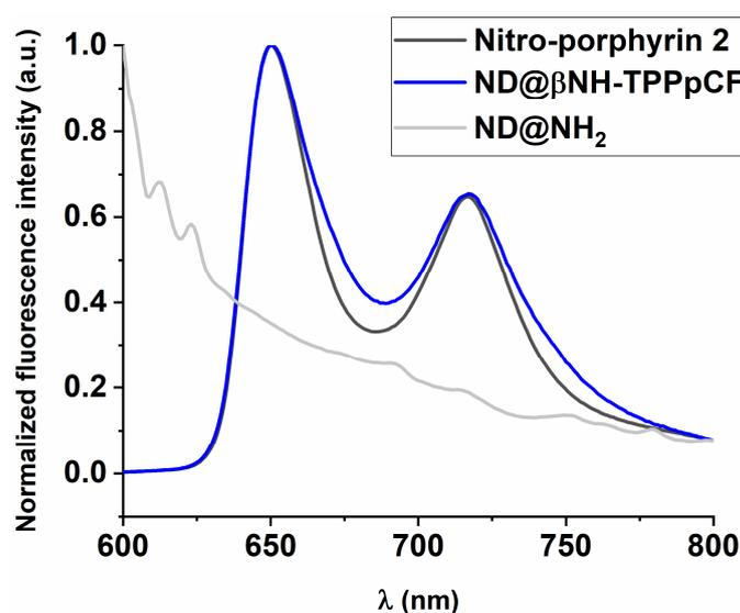
**Figure 1.** Normalized fluorescence emission spectra of ND@βNH-TPPpCF<sub>3</sub> (blue line), ND@NH<sub>2</sub> (grey line), and nitro-porphyrin **2** (black line) in DMF with excitation at 420 nm.
