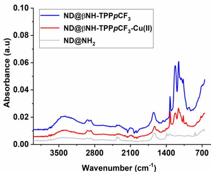
**Figure 3.** FT-IR spectra of ND@NH<sub>2</sub> (grey line), ND@βNH-TPPpCF<sub>3</sub>-Cu(II) (red line) and ND@βNH-TPPpCF<sub>3</sub> (blue line).
