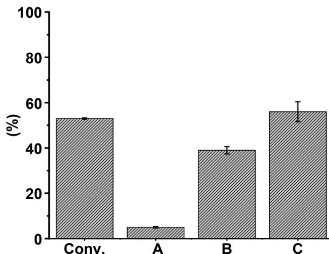
**Figure 4.** Conversion of cyclohexene (%) and product selectivity (%) (A = 1,2-epoxycyclohexane; B = cyclohexen-1-one; C = 2-cyclohexen-1-ol) when using ND@ $\beta$ NH-TPP $p$ CF<sub>3</sub>-Cu(II) as catalyst.
