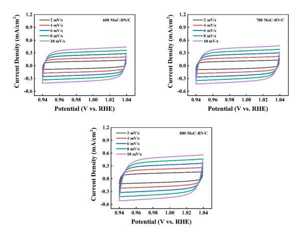
Figure S3. CV graphs of 600, 700, and 800 MoC-BN/C to identify the electrochemically active surface area
