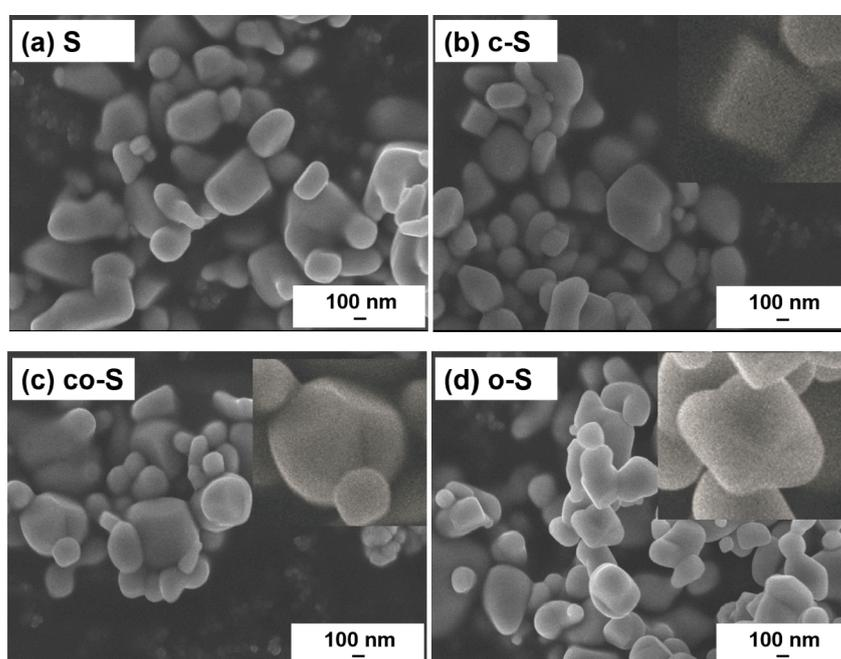
Figure S1. SEM images of titania and FCP-loaded titania synthesized at 328 K.
