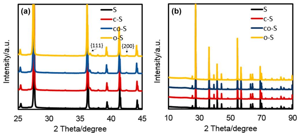
Figure S4. XRD patterns of titania (ST-G2) and FCP-loaded titania. (a) is the zoom-in XRD patterns between 25° to 45 °.
