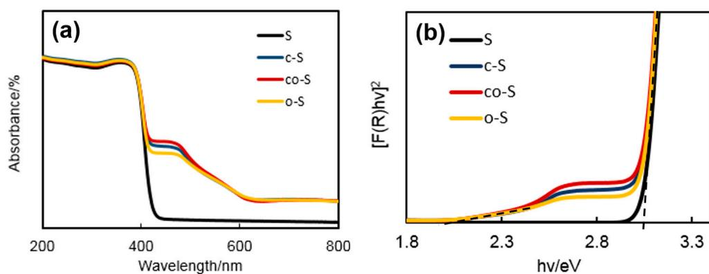
Figure S5. (a) Diffuse reflectance spectra and (b) Tauc plots with Kubelka–Munk function derived from reflection spectra of titania (ST-G2) and FCP-loaded titania.
