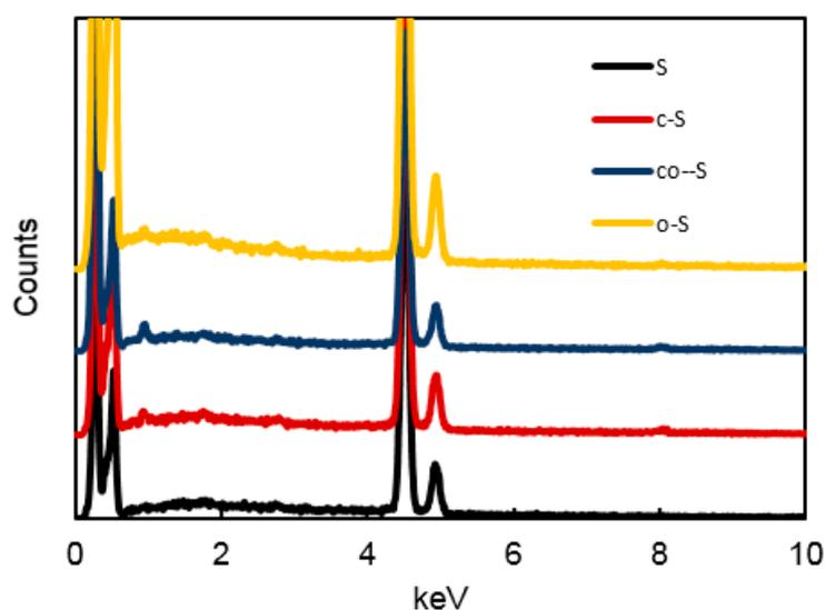
Figure S3. EDS spectra of titania and FCP-loaded titania synthesized at 328 K.
