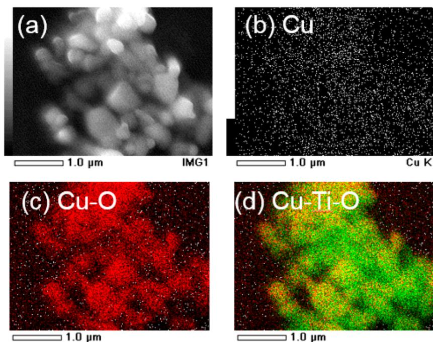
Figure S2. SEM images and EDS mapping results of o-S.
