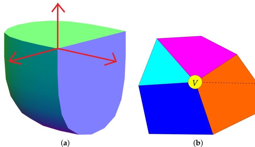
**Figure 6.** (a) Multiple normals associated with sharp vertices. (b) Regions (in different colours) separated by sharp edges (black solid lines) and non-sharp edges (black dashed lines).
