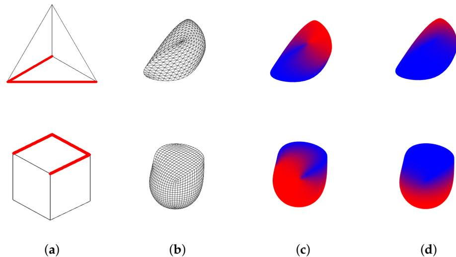
**Figure 5.** Top row: A tetrahedron model with two sharp edges (red) with sharpness value 4. Bottom row: A cube model with three sharp edges (red) with sharpness value 4. From left to right: (a) The control mesh with sharp edges highlighted. (b) The control mesh after 4 subdivision steps. (c) The blending weights when darts are treated as smooth vertices. (d) The blending weights when darts are treated as sharp vertices.
