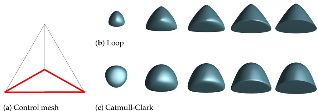
**Figure 1.** A tetrahedron (a) with three sharp edges (red) all with sharpness values  $s$  after six subdivision steps. The top row (b) shows Loop subdivision, and the bottom row (c) illustrates Catmull-Clark subdivision. From left to right:  $s = 0, s = 1, s = 2, s = 4, s = 6$ .
