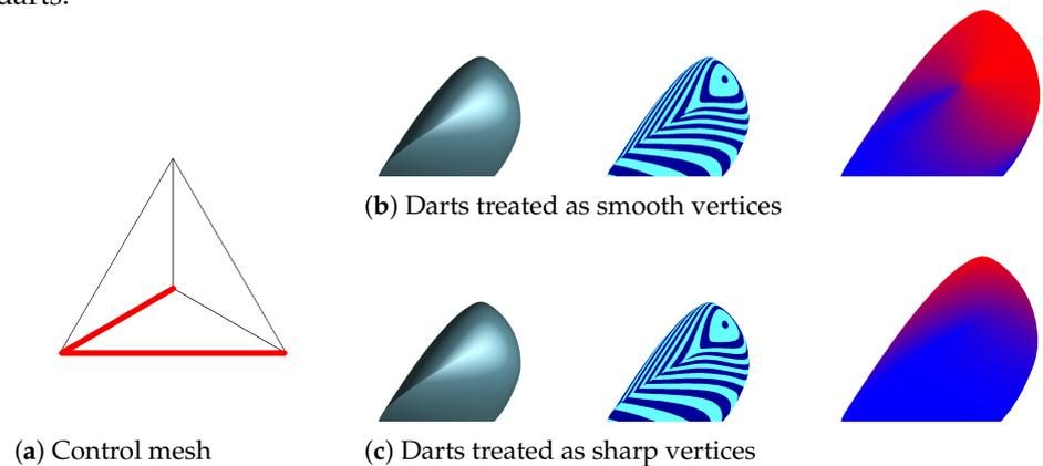
**Figure 12.** (a) The tetrahedron model with two sharp edges. We show the difference between treating darts as smooth vertices (b) or as sharp vertices (c) when setting the blend weights.
