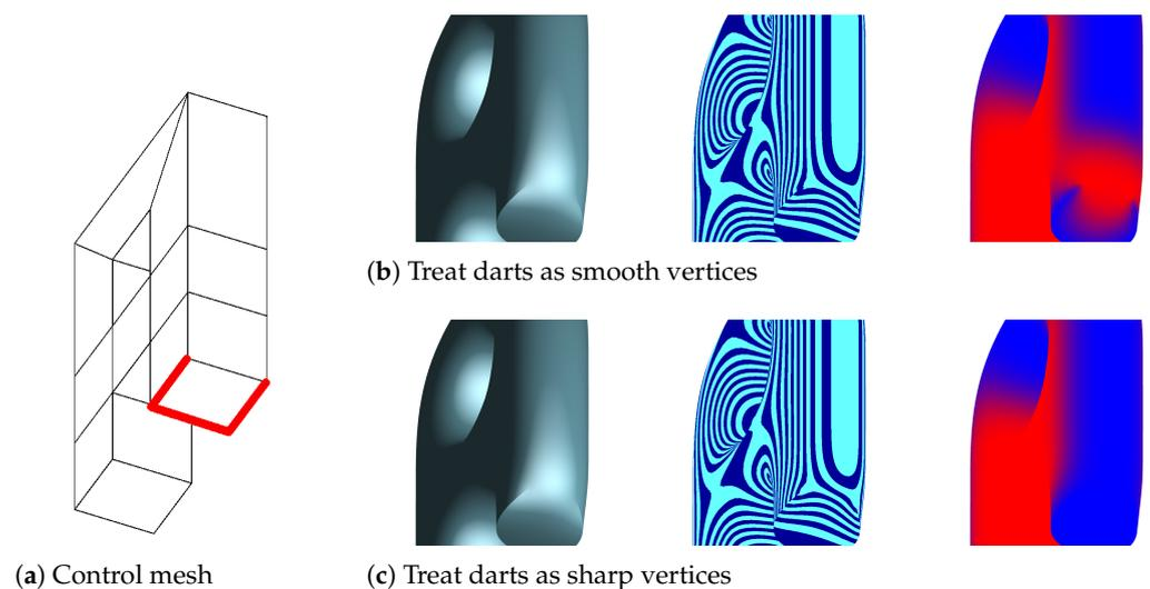
**Figure 13.** (a) The Letter A model with three sharp edges. We show the difference between treating darts as regular vertices (b) or as sharp vertices (c) when setting the blend weights.
