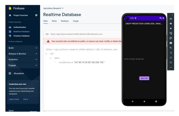
Figure 3. Firebase real-time cloud database connected with Android application.
