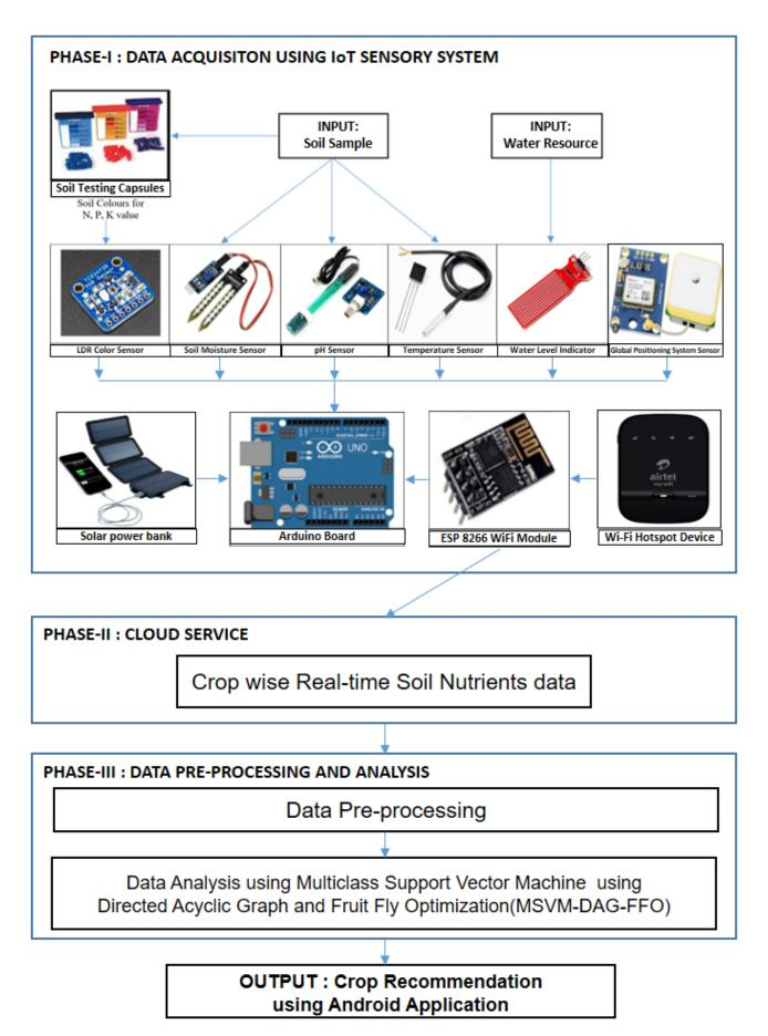
Figure 1. Proposed model for IoT-enabled soil nutrient analysis and crop recommendation.
