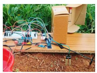
(b) Sensor connectivity using Arduino
