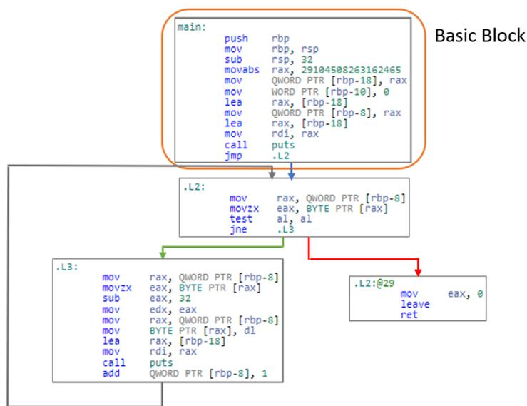
Figure 1. Control Flow Graph.
