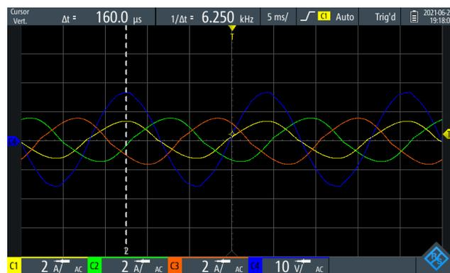
Figure 11. Three-phase resistive load profile.
