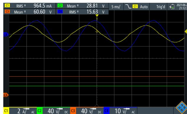
Figure 13. Resistive-capacitive load profile and DC voltages.
