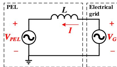
Figure 1. PEL operation principle.
