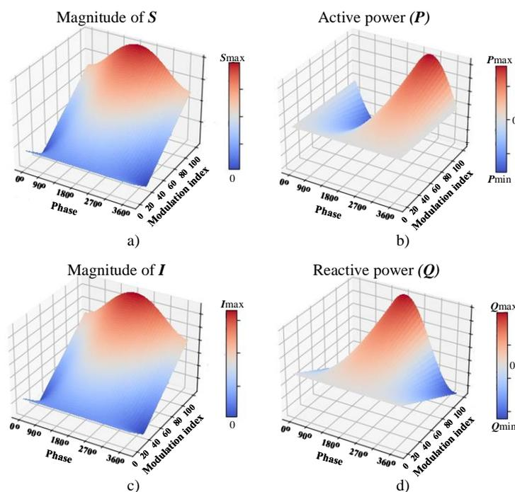
**Figure 6.** Operation modes of the PEL: A 3D representation. (a) magnitude of  $S$ , (b) active power, (c) magnitude of  $I$ , (d) reactive power
