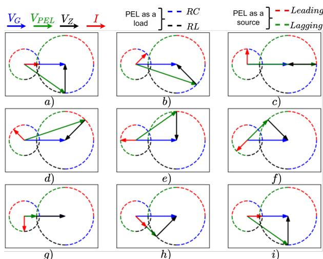
**Figure 3.** Operation modes of the PEL:  $|I| = |I_{max}|$  with  $0^\circ \leq \theta_I < 360^\circ$ . (a) pure resistive load, (b) resistive-capacitive load, (c) capacitive load, (d) leading source, (e) pure active source, (f) lagging source, (g) pure lagging source, (h) resistive-inductive load, (i) pure resistive load.
