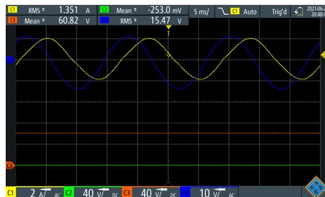
Figure 14. Inductive load profile and DC voltages.
