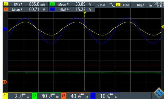
Figure 15. Resistive load profile and DC voltages.
