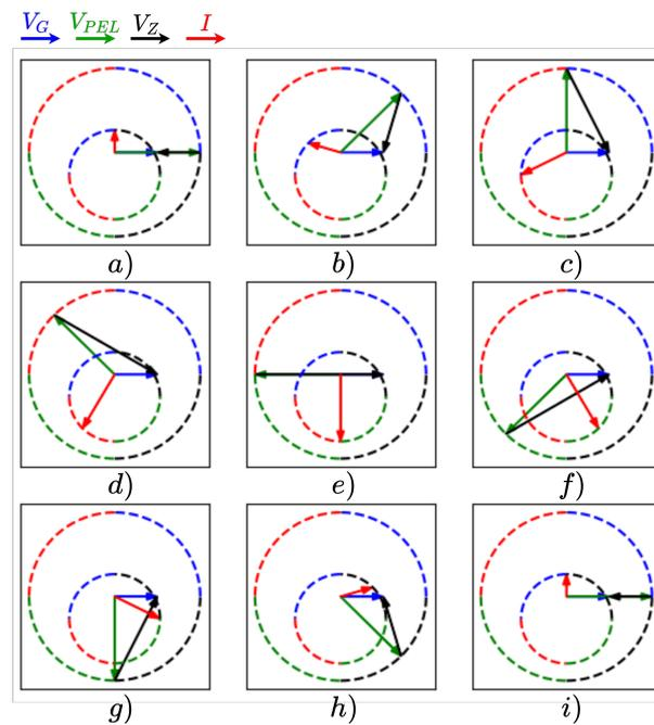
**Figure 4.** Operation modes of the PEL:  $|V_{PEL}| = |V_G|$  with  $0^\circ \leq \theta_{PEL} < 360^\circ$ . (a) pure resistive load, (b) resistive-capacitive load, (c) capacitive load, (d) leading source, (e) pure active source, (f) lagging source, (g) pure lagging source, (h) resistive-inductive load, (i) pure resistive load.
