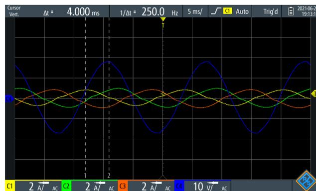
Figure 12. Three-phase capacitive load profile.
