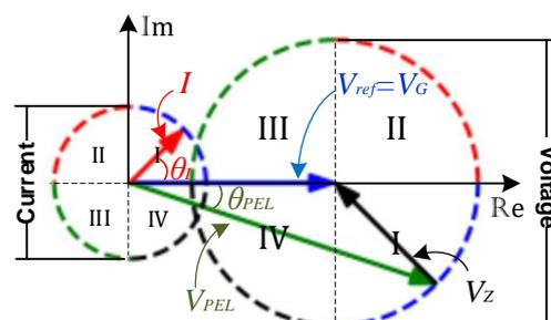
Figure 2. Phasor diagram of the PEL current and voltages path.
