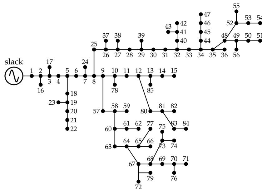
Figure 2. Electrical configuration of the IEEE 85-bus grid.
