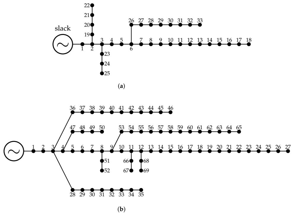
Figure 1. Test feeder grid configuration: (a) IEEE 33- and (b) IEEE 69-node system.
