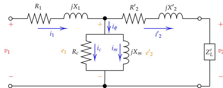
**Figure 1.** Transformer equivalent circuit referred to the primary side.
