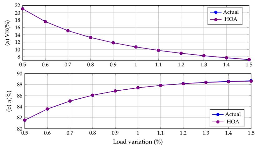
**Figure 3.** Behavior of the 10 kVA test transformer with load variations: (a) Voltage regulation and (b) Efficiency.
