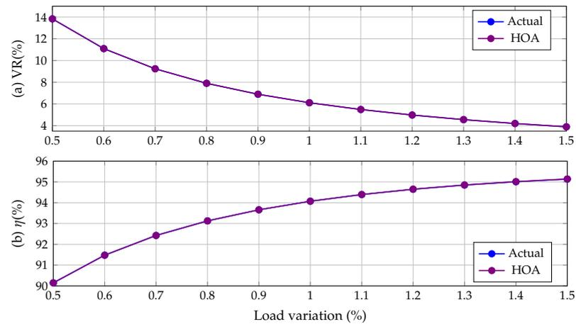
**Figure 2.** Behavior of the 4 kVA test transformer with load variations: (a) Voltage regulation and (b) Efficiency.
