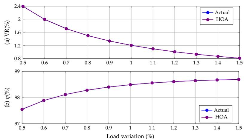
**Figure 4.** Behavior of the 15 kVA test transformer with load variations: (a) Voltage regulation and (b) Efficiency.
