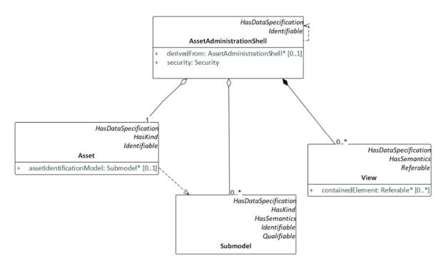
Figure 2. Excerpt from the AAS meta-model. Adapted from ref. [15].
