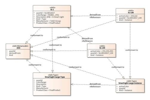
Figure 11. Instance and type information according to the AAS specification [15].
