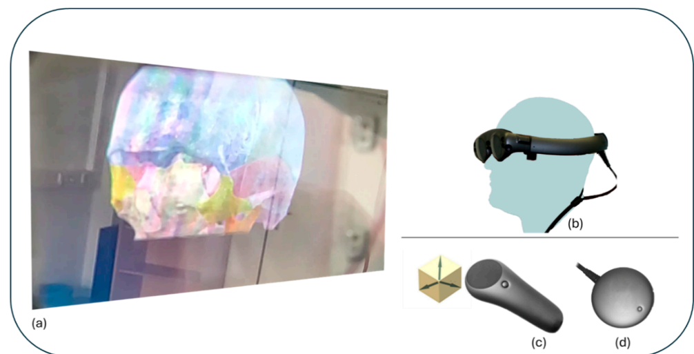
Figure 2. Magic Leap 1 Device (Plantation, FL, USA): (a) Visualisation of the immersive MR content. (b) Head-Mounted Display. (c) 6 DoF Controller. (d) Compute Pack.
