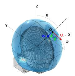
**Figure 4.** Reference schematic for the arrangement of a single antenna. Note that the angle  $\phi$ , while following the classic right-hand convention, is shown here on the negative *y* half-space for readability. The figure refers to a local coordinate system centered at the ellipsoid's center and aligned with the global cartesian axes.
