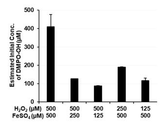
**Figure 8.** Estimation of the initial concentration of •OH generated by the Fenton reaction. Columns and error bars indicate the average and SD of 3 experiments.
