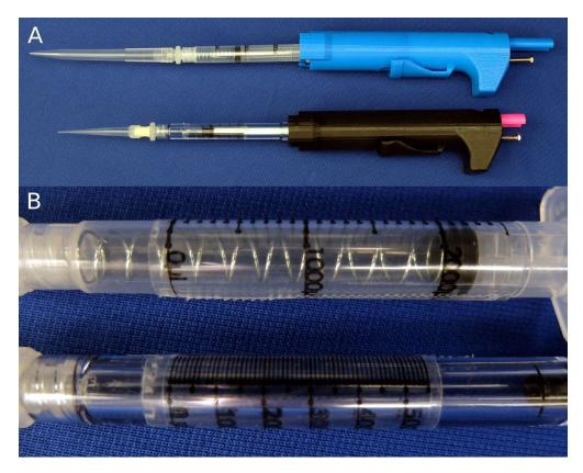
**Figure 4.** Photos of assembled pipettes. **(A)** Two assemblies of the pipette: the 100–1000-µL configuration (top) and the 30–300-µL configuration (bottom). **(B)** Close-up photo of the taped on scale for each of the syringes. Scales are available in the Appendix A: Figures A1 and A2.
