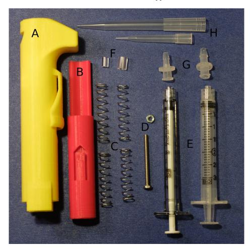
**Figure 3.** Photo of the parts to make the pipette. (**A**) Printed body part. (**B**) Printed plunger part. (**C**) Springs. (**D**) M3 hex nut and M3 bolt. (**E**) Disposable syringes. (**F**) Two sizes of tubing to adapt pipette tips to luer barbs. (**G**) Luer lock syringe-to-barb adapters. (**H**) Pipette tips. A list of parts is in Appendix A: Tables A1 and A2.
