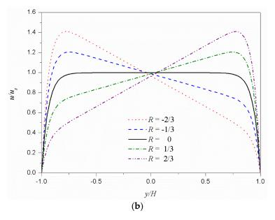
**Figure 4.** Dimensionless velocity distributions  $u/u_s$  as a function of the dimensionless zeta potential difference *R*. The values -2/3, -1/3, 0, 1/3, and 2/3 of *R*, correspond to 0.2, 0.5, 1.0, 2.0, and 5.0 of the zeta potential ratio ( $\psi_t/\psi_b$ ), respectively. (**a**) Shear thinning fluid (n = 0.8). (**b**) Shear thickening fluid (n = 1.2).
