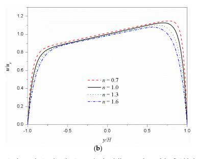
**Figure 2.** Dimensionless velocity distributions  $u/u_s$  for different values of the fluid behavior index *n* under  $\kappa H = 15$ . (a) Symmetric zeta potentials ( $\psi_t/\psi_b = 1$ ). (b) Asymmetric zeta potentials ( $\psi_t/\psi_b = 1.5$ ).
