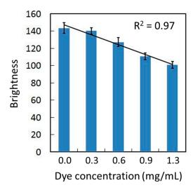
**Figure S1.** Calibration between dye concentration and brightness. The brightness of the colored water using the dye is linear in the range of our usage. The R-squared value is 0.97 when the data is linearly fitted.
