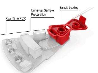
**Figure 1.** Schematic description of the GenePOC disposable, a MCD integrating the essential functions and components for performing nucleic acid-based diagnostics at POC. Copyright © GenePOC Inc. 2016 All rights reserved.
