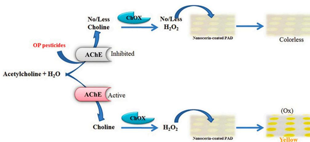
**Figure 3.** Colorimetric detection of pesticides based on the enzyme inhibition properties of the pesticide on nanoceria substrate. Reprinted with permission from reference [42]. Copyright 2016 The Royal Society of Chemistry.
