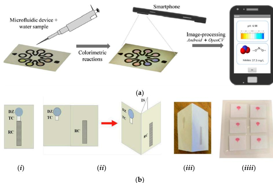
**Figure 4.** (a) Griess-color reaction assay-based detection methods for nitrite using a smartphone for image processing. Reprinted with permission from reference [45]. Copyright 2014 American Chemical Society. (b) Griess-color reaction assay-based detection methods for nitrite and nitrate using 2D (i) and 3D (ii–iv)  $\mu$ PADs. Reprinted with permission from reference [53]. Copyright 2014 American Chemical Society.
