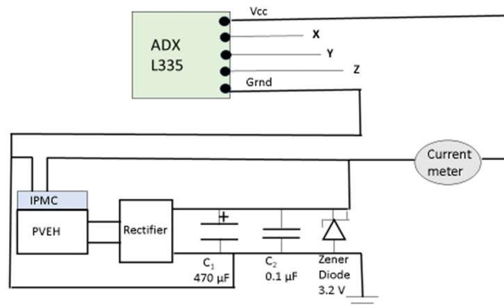
**Figure 6.** Circuit for powering the MEMS accelerometer and IPMC using PVEH output.
