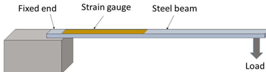
**Figure 4.** Experimental setup of the strain-gauged beam.
