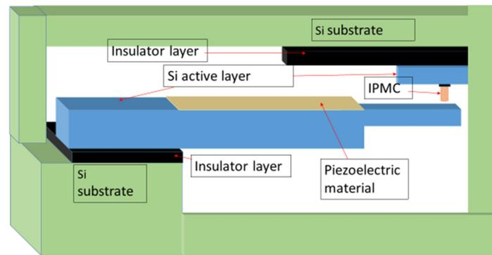
**Figure 10.** MEMS scheme for the novel design of tunable PVEH based on the SOI process.
