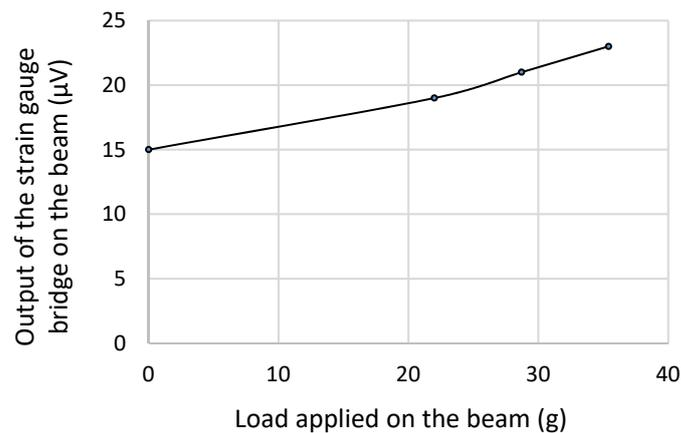
**Figure 9.** Response of the strain gauge bridge powered by the harvester.
