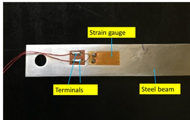
**Figure 3.** Steel beam with a strain gauge bonded to it.
