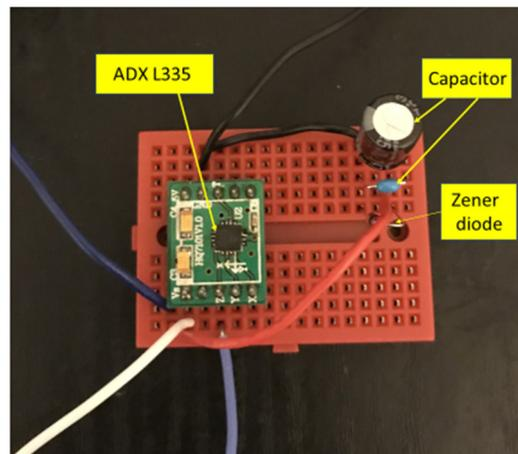
**Figure 5.** ADX L335 MEMS accelerometer and circuit.
