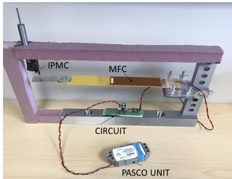
Figure 7. Setup of the PVEH powering the PASCO Bluetooth device.
