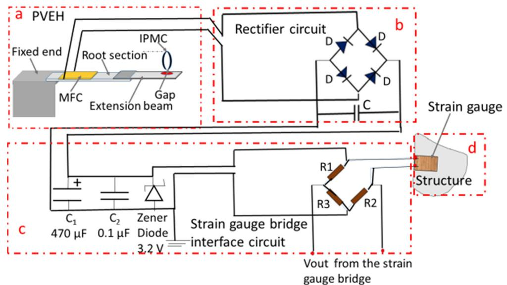
**Figure 2.** Circuit for powering a strain gauge bridge using the PVEH output. (a) PVEH; (b) Rectifier circuit; (c) Strain gauge bridge interface circuit; (d) Structure on which strain gauge is fixed.
