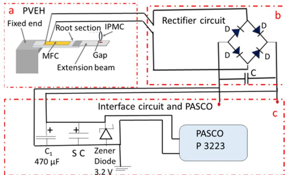
Figure 8. Circuit of the setup for powering the PASCO accelerometer/transmitter unit. (a) PVEH; (b) Rectifier circuit; (c) Interface circuit and PASCO unit.
