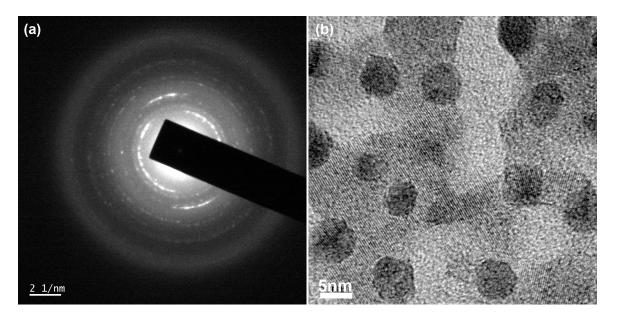
**Figure 7.** (a) Selected area diffraction pattern and (b) high-resolution TEM image of the self-doped CsPbI<sub>3</sub> sample.
