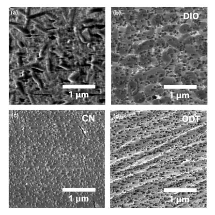
**Figure 9.** SEM images: (a) self-doped CsPbI<sub>3</sub>, (b) self-doped CsPbI<sub>3</sub> with DIO, (c) self-doped CsPbI<sub>3</sub> with CN, and (d) self-doped CsPbI<sub>3</sub> with ODT.
