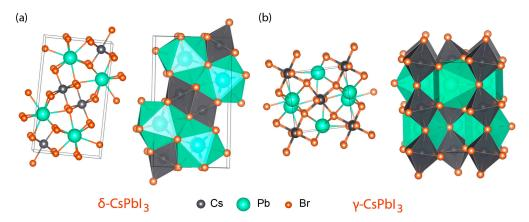
**Figure 3.** Crystal structures of (a) yellow  $\delta$ -phase CsPbI<sub>3</sub> and (b) black  $\gamma$ -phase CsPbI<sub>3</sub>.
