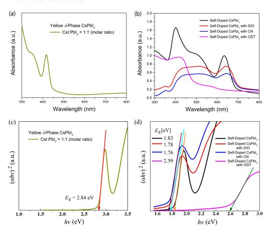
**Figure 5.** UV-vis absorption spectra of (a) yellow  $\delta$ -phase CsPbI<sub>3</sub> and (b) black  $\gamma$ -phase CsPbI<sub>3</sub> and its derivative (e.g., Cs<sub>4</sub>PbI<sub>6</sub> or low dimensional structure). Tauc plot for determining bandgap of (c) yellow  $\delta$ -phase CsPbI<sub>3</sub> and (d) black  $\gamma$ -phase CsPbI<sub>3</sub> and its derivative. Here, the arrows indicate a tangential line to determine the optical bandgap.
