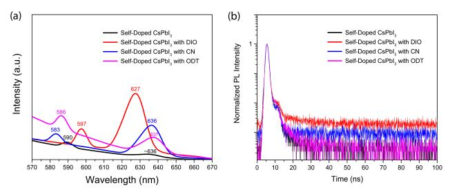
**Figure 6.** Self-doped CsPbI<sub>3</sub> without/with organic additive: (a) PL emission spectra and (b) time-resolved PL decay spectra.
