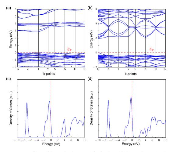
**Figure 4.** Electronic band structures: (a) yellow δ-phase CsPbI<sub>3</sub> with the energy bandgap,  $E_g = 2.87$  eV and (b) black  $\gamma$ -phase CsPbI<sub>3</sub> with  $E_g = 1.90$  eV. Density of states: (c) yellow δ-phase CsPbI<sub>3</sub> and (d) black  $\gamma$ -phase CsPbI<sub>3</sub>. Here,  $E_F$  stands for Fermi energy. Here, the red dot line is y = 0 for (a) and (b) and x = 0 for (c) and (d), respectively.
