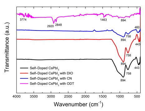
Figure 10. FTIR spectra of self-doped CsPbI<sub>3</sub> without and with organic additives, DIO, CN, and ODT.
