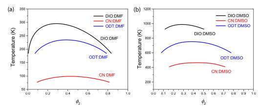
**Figure 2.** Phase diagrams of binary additive–solvent systems: (a) additive–DMF system and (b) additive–DMSO system. Here, the additive could be DIO, CN, or ODT, which has a molar volume with oligomer level compared to typical solvents such as DMF and DMSO.
