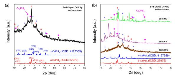
Figure 8. XRD patterns for (a) self-doped CsPbI<sub>3</sub> without organic additive and (b) self-doped CsPbI<sub>3</sub> with organic additives such as DIO (brown), CN (violet), and ODT (green). Note that the blue solid line is for  $\gamma$ -CsPbI<sub>3</sub> from the Inorganic Crystal Structure Database (ICSD-4127359) whereas the red solid line is for δ-CsPbI<sub>3</sub> from ICSD-27979. The pink filled circles indicate the XRD peaks from the trigonal Cs<sub>4</sub>PbI<sub>6</sub> phase [95].
