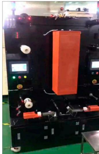
**Figure 6.** Nano-coating device for micro wire surface [34]. Reproduced with permission from ref. [34]; published by The Chinese Journal of Nonferrous Metals, 2020.
