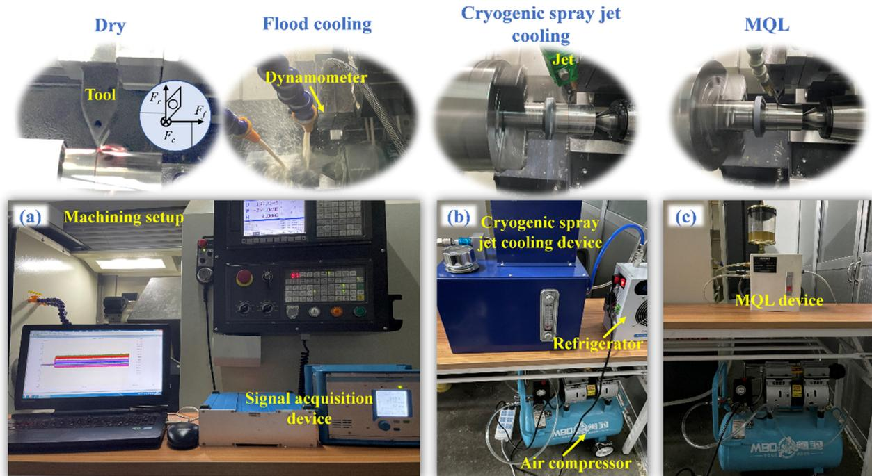
**Figure 4.** Turning procedure of Ti-6Al-4V under dry and three types of cooling conditions. (a) Turning experimental set-up. (b) CSJC device. (c) MQL device.
