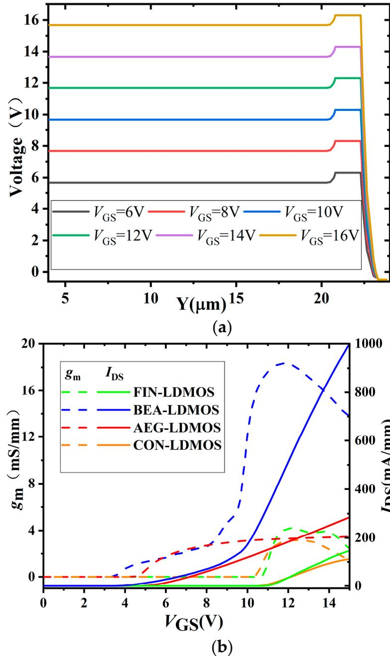
**Figure 3.** The gate potential  $V_{GS}$  in the on-state, transfer, and  $g_m$  characteristics for the devices. (a) Potential distribution along the p-n-p for the BEA-LDMOS. (b) Transfer and  $g_m$  of the CON-LDMOS, FIN-LDMOS, AEG-LDMOS, and BEA-LDMOS.
