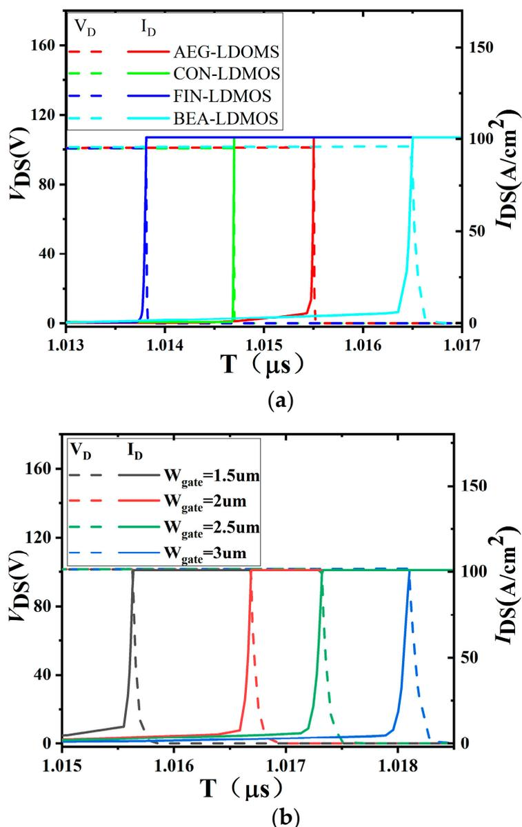
Figure 11. (a) Capacitance switching characteristics of the four devices. Turn-on and turn-off curves under inductive load. (b) Switching characteristic curves at different gate widths.
