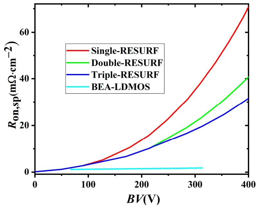
**Figure 12.** The trade-off relationship between  $R_{on,sp}$  and  $BV$  for the BEA-LDMOSs and the RESURF. The FOM is calculated by the  $FOM = BV^2/R_{on,sp}$ .
