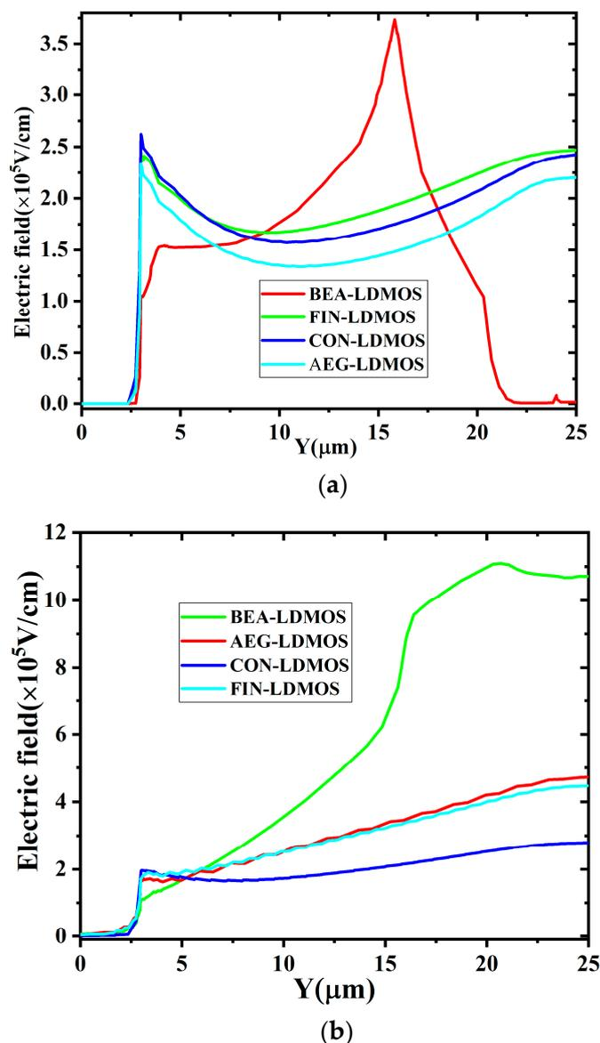
**Figure 9.** The electric field distribution at the avalanche breakdown at (a)  $X = 1.9 \mu\text{m}$ ,  $Z = 6 \mu\text{m}$ ; (b)  $X = 1.9 \mu\text{m}$ ,  $Z = 4.9 \mu\text{m}$ .
