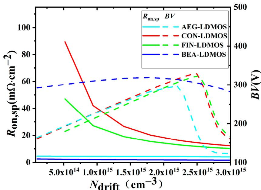
Figure 7. Effect of doping concentration of N-drift region on BV and  $R_{on,sp}$  for the four devices.
