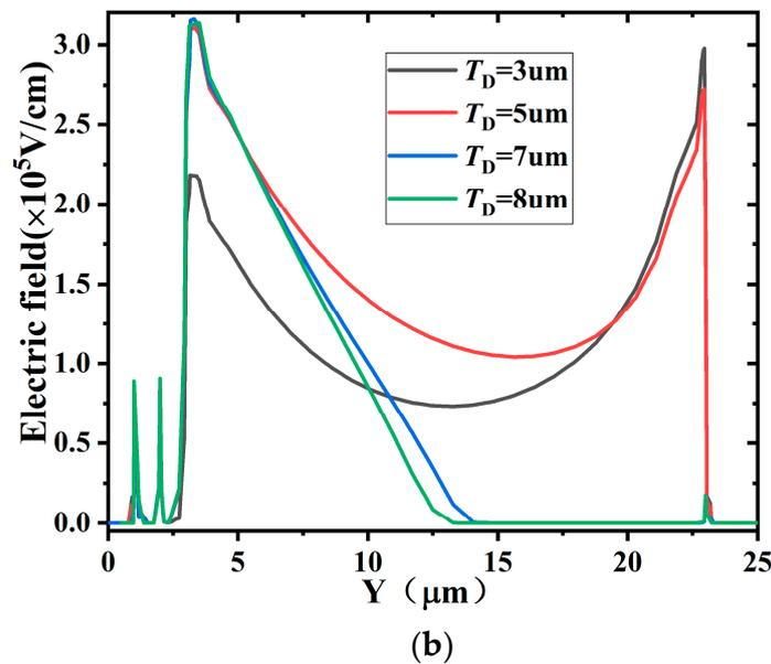
**Figure 6.** Influence of key parameter  $T_D$  on the  $R_{on,sp}$ ,  $BV$ , and electric field for the BEA-LDMOS ( $T_D$  is the thickness of the N-drift). (a) Influence on the  $R_{on,sp}$  and  $BV$ , (b) influence on the electric field of top layer.
