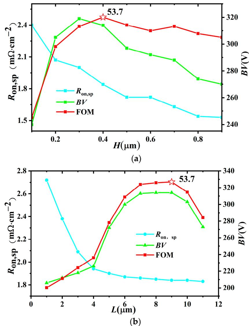
Figure 10. Key parameters: (a) thickness ( $H$ ) of the Extended Drain, (b) length ( $L$ ) influence on the  $R_{on,sp}$ , peak  $g_m$ , and  $BV$  for the BEA-LDMOS.
