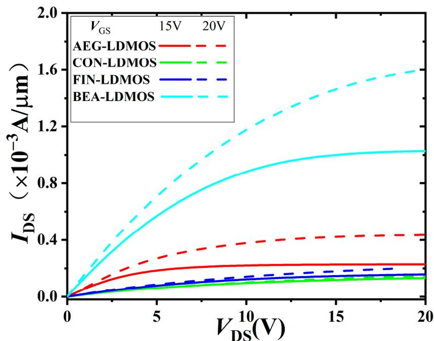
Figure 5. Output characteristics of the devices, and  $V_{GS}$  of 15 and 20 V are applied.
