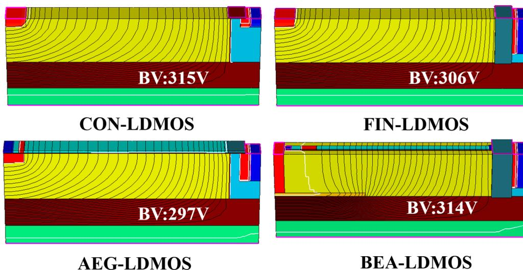
Figure 8. The 3-D equipotential contours at the avalanche breakdown at the same  $N_{drift}$ .
