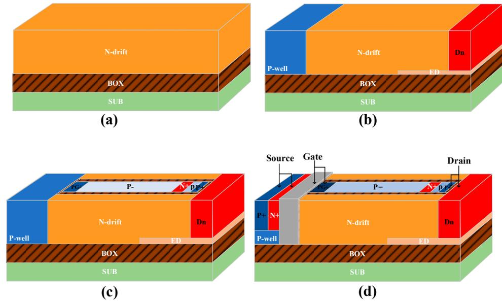
**Figure 2.** Simplified key process of the proposed BEA-LDMOS. (a) SOI substate, (b) Ion doping, (c) Thermal oxidation, (d) Electrode deposition.
