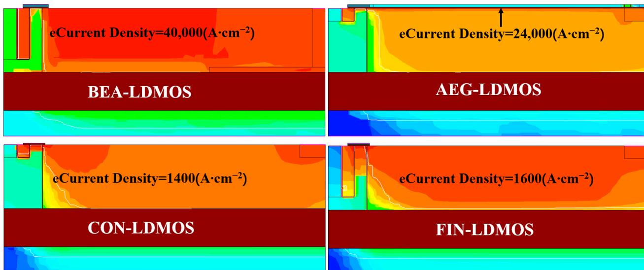
Figure 4. The electron Current density distribution for the four devices at the On-state.
