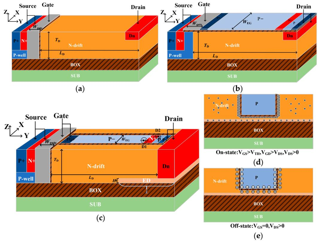
**Figure 1.** The three-dimensional (3D) schematic and mechanism of the three proposed devices. (a) FIN-LDMOS, (b) AEG-LDMOS, (c) BEA-LDMOS, (d) the Bulk Electron Accumulation (BEA) effect induced at the N-drift, (e) the assisted depletion between the P-region and N-drift in the Off-state. Diode D1 is formed by the (P−/N+) and D2 is formed by the (P/N+) junction.
