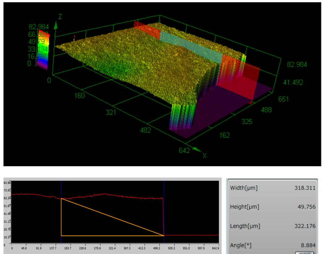
**Figure 5.** Thickness measurement of the graphene-chitin film.
