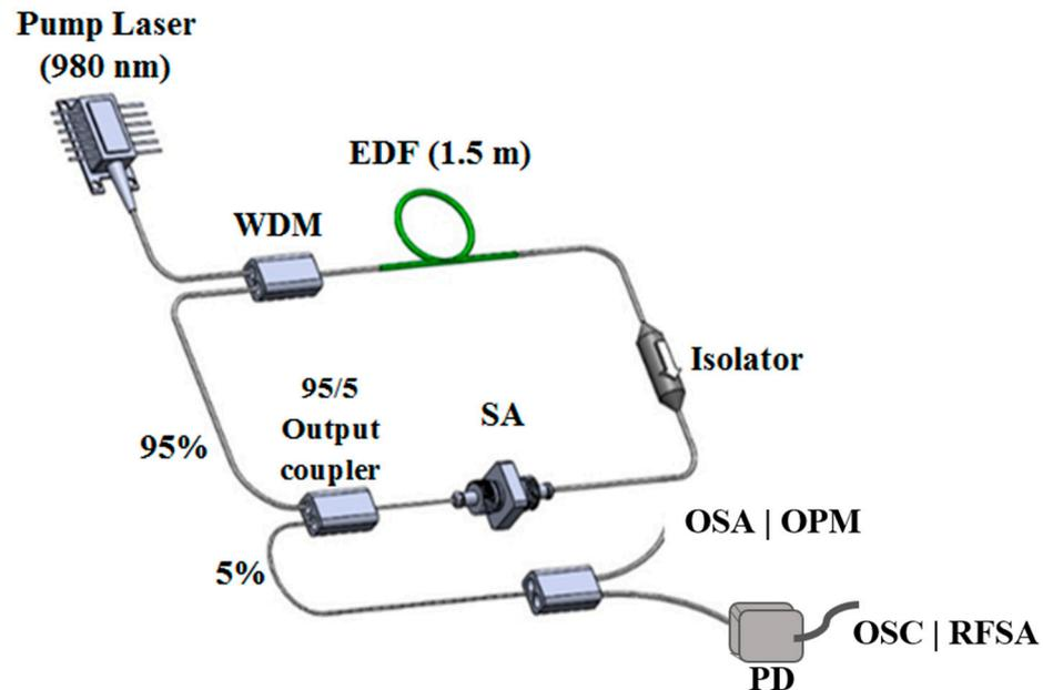
Figure 7. Experimental setup of EDFL incorporating graphene-chitin film-based SA.
