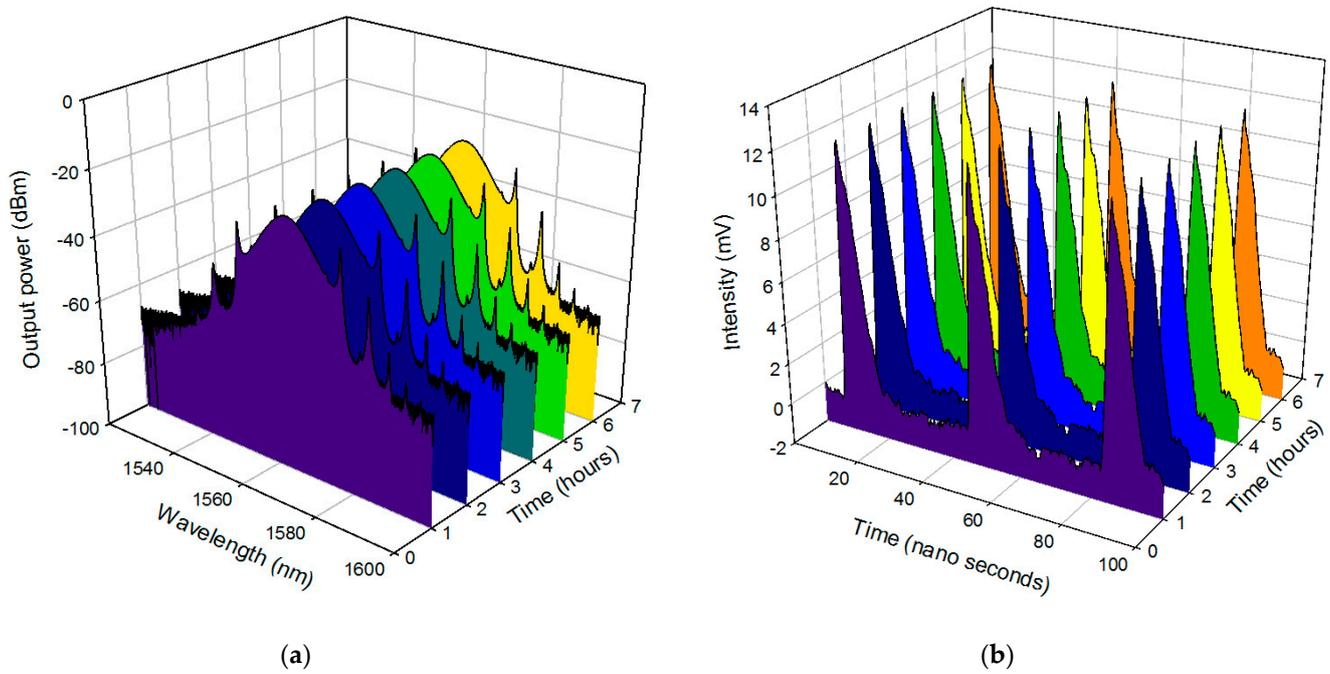
**Figure 16.** The stability of the output spectrum for graphene-chitin based SA as passive mode locker over 6 h at a 1-h interval.
