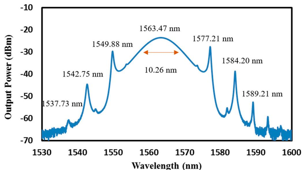
**Figure 13.** Optical spectrum of the soliton mode-locked EDFL based on graphene–chitin film.
