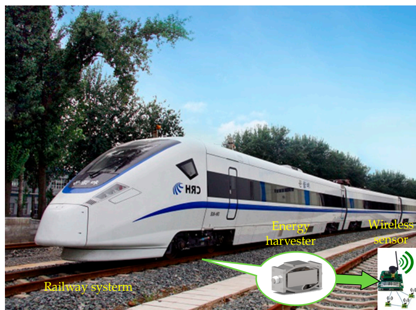
Figure 1. Schematic diagram of vibration energy harvesting system applied to railway track.
