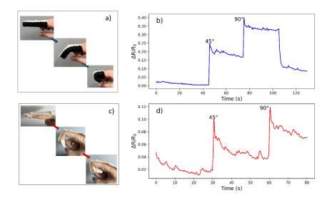
**Figure 5.** The relative resistance change versus time for Version 1 and Version 2 at various positions: relaxation, 45° and 90°. (a) The positions of version 1 sensors at different angles, (b) relative resistance changes versus time of version 1 sensor, (c) the positions of the Version 2 sensor at different angles, and (d) relative resistance changes versus time of the Version 2 sensor.
