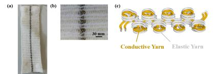
**Figure 1.** (a) The developed knitted strain sensor, (b) optical images of the sensing region which shows the conductive yarns (gold) positioned inside and elastic yarns outside (white), and (c) illustration of the conductive and elastic yarn positioning within the sensing region.
