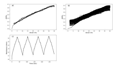
**Figure 3.** The developed knitted strain sensor graphs under four cyclic tests, (**a**) Relative resistance change versus strain, (**b**) Relative resistance change versus strain for 70 repetitive cycles, and (**c**) Resistance changes versus time at a strain 40% strain under 4 cycles.
