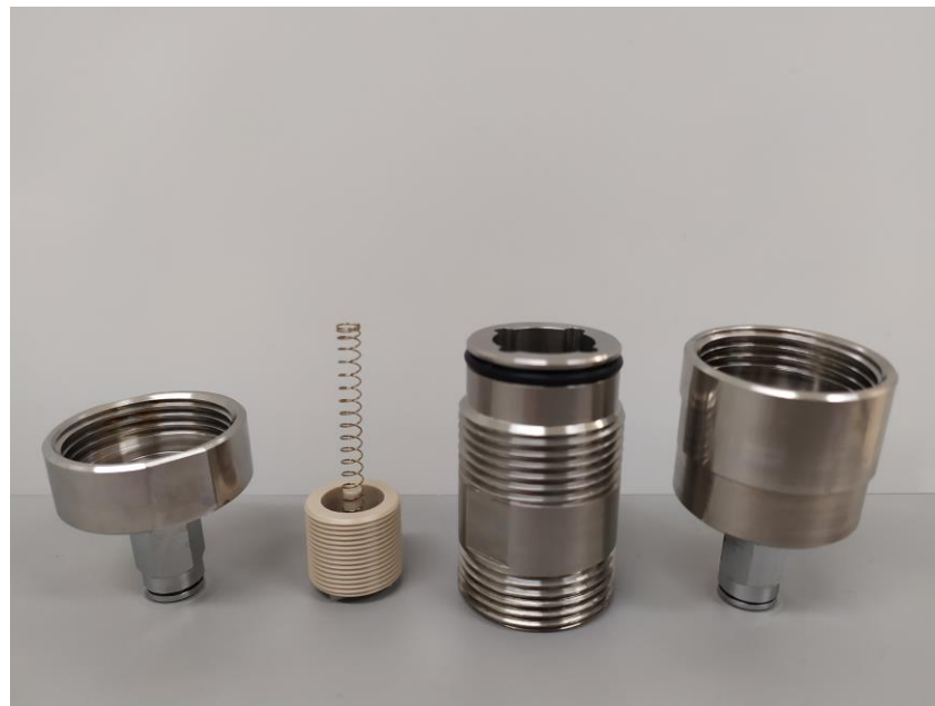
Figure 5. Prototype teardown showing, from left to right: the inlet flange, the piston, and the spring, the cylinder, and the outlet flange. Nominal dimensions are provided in the mechanical drawings. The height of the piston made of PEEK is 2 mm shorter than expected and the clearance between the piston and the cylinder is larger than expected (inner diameter of the cylinder at 18.035 mm instead of 18.015 mm); the other parts are within specification.
