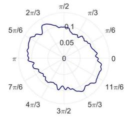
Figure 14. Radial error of the spindle.
