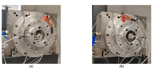
Figure 10. Donaldson reversal method measurement device: (a) before reversal, (b) after reversal.
