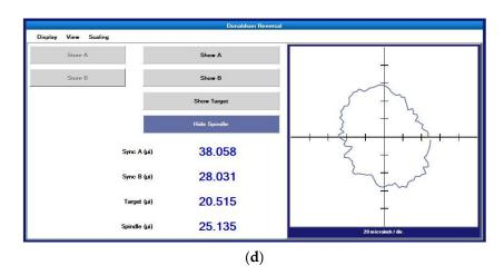
**Figure 11.** Donaldson reversal method measurement data: (**a**) synchronization error before reversal, (**b**) synchronization error after reversal, (**c**) roundness error of standard workpiece, (**d**) spindle radial error.
