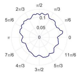
Figure 15. Roundness error of the standard workpiece.
