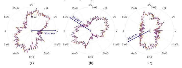
**Figure 12.** Amplitude phase diagrams of the multi-turn sampling data of the three sensors with the eccentricity and synchronization error removed in the polar coordinate system: (a) data from sensor A, (b) data from sensor B, and (c) data from sensor C.
