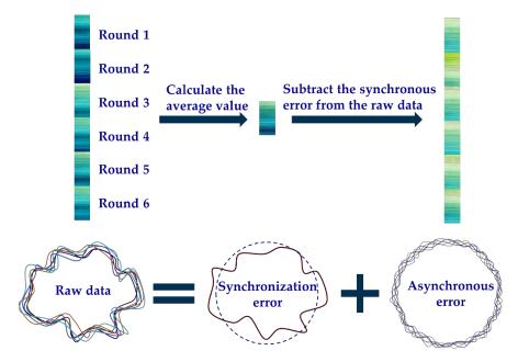
Figure 2. Separation of synchronous and asynchronous errors.
