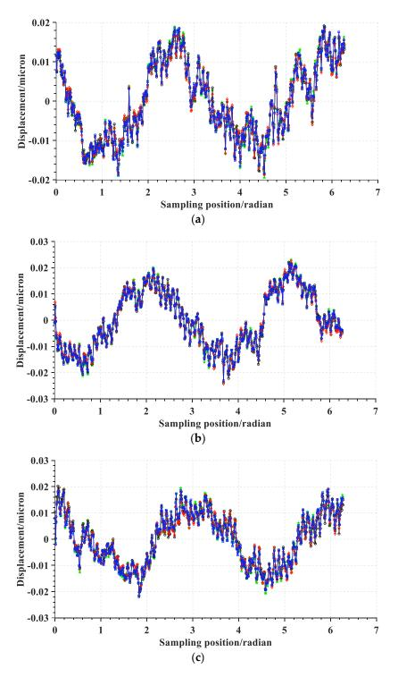
**Figure 13.** Amplitude phase diagrams of the multi-turn sampling data of the three sensors with the eccentricity and synchronization error removed in the Cartesian coordinate system: (**a**) data from sensor A, (**b**) data from sensor B, and (**c**) data from sensor C.
