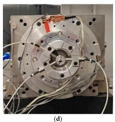
**Figure 9.** Detailed steps of radial error measurement using three-point method: (**a**) step 1: mounting of standard workpiece, (**b**) step 2: rough adjustment of standard workpiece, (**c**) step 3: fine adjustment of standard workpiece, (**d**) step 4: mounting fixture and sensor probes.
