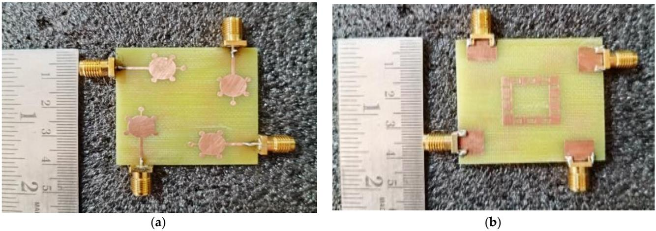
Figure 10. Fabricated prototype model of proposed spike antenna (a) front view, (b) back view.
