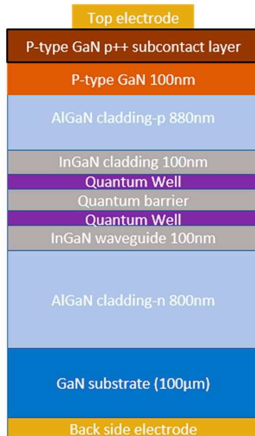
Figure 1. Schematic cross-section of the epitaxial structure of laser diodes used in the present study [20].
