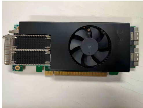
Figure 5. TCP Offload Engine (TOE) on FPGA chip.
