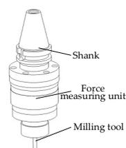
**Figure 4.** Milling force-measurement tool system for the cross-beam structure.
