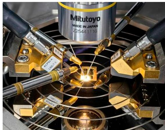
**Figure 2.** On-wafer measurement setup.
