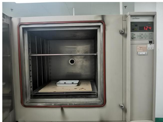
**Figure 9.** High-temperature accelerated test chamber.
