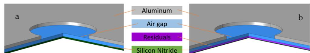
**Figure 8.** Designed and produced sizes of mirrors. (a) Designed mirrors: radius 35/45  $\mu\text{m}$ , silicon nitride thickness = 200 nm, no HF residuals; (b) Fabricated mirrors: radius 37/42  $\mu\text{m}$ , silicon nitride thickness = 60 nm, residuals height = 180 nm.
