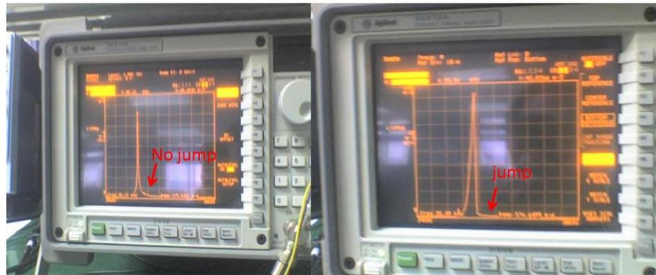
**Figure 22.** Nonlinear characteristics of the accelerometer.
