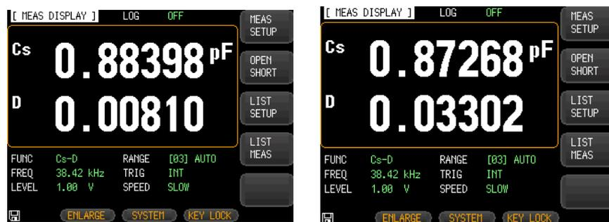
Figure 14. Interface capacitance test (driving capacitance).
