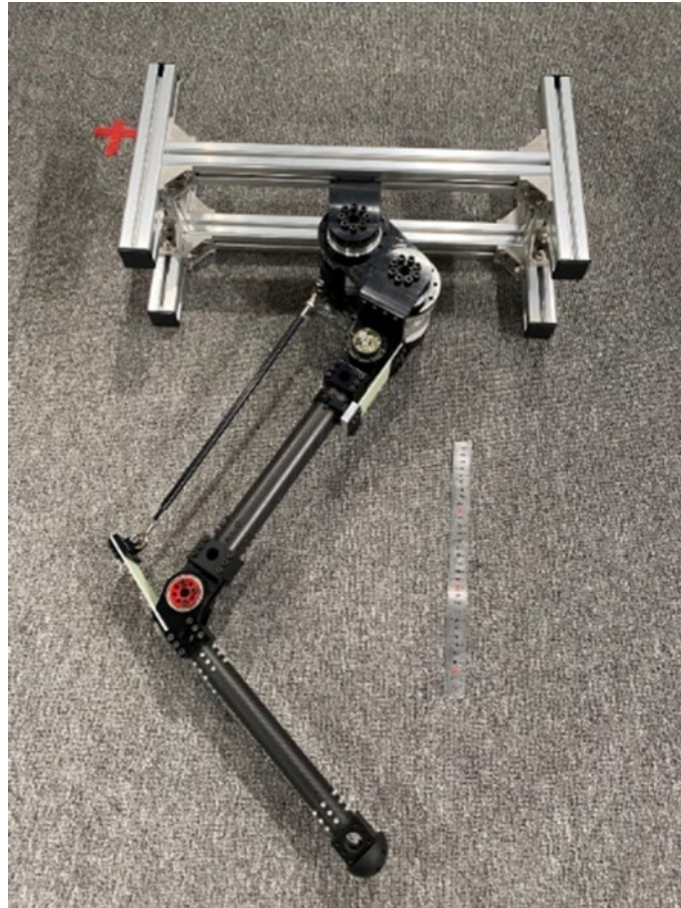
Figure 1. The compliant one-legged robot which was designed by ourselves.
