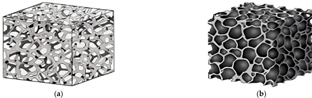
**Figure 13.** (a) Open pores of ceramic material; (b) Closed pores of ceramic material (Reprinted from Ref. [84], copyright (2007), with the kind permission of American Chemical Society).
