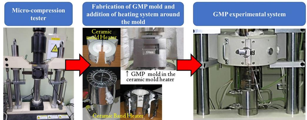
Figure 14. GMP experimental system for 2-step glass molding process.
