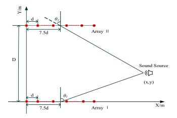
Figure 4. Sound source and microphone array simulation location.
