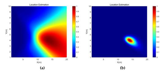
**Figure 6.** The location estimation simulation results of (a) SRP-PHAT and (b) SRP-MCCC when the SNR is -5 dB.
