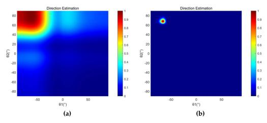
**Figure 8.** The direction estimation experimental results of (**a**) SRP-PHAT and (**b**) SRP-MCCC when the sound source coordinate is (10, 5).
