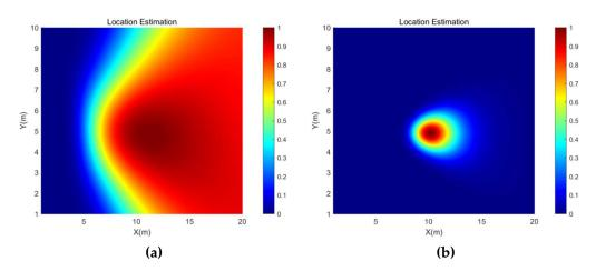
**Figure 9.** The location estimation experimental results of (a) SRP-PHAT and (b) SRP-MCCC when the sound source coordinate is (10, 5).
