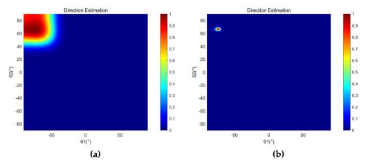
**Figure 5.** The direction estimation simulation results of (a) SRP-PHAT and (b) SRP-MCCC when the SNR is -5 dB.
