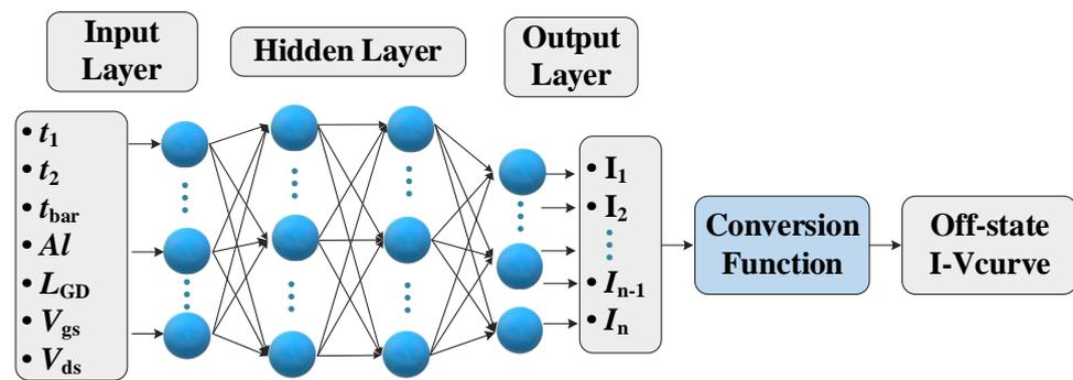
Figure 3. The overall flow of the proposed framework for off-state performance characterization.
