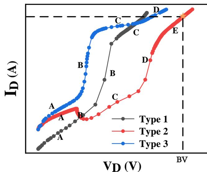
**Figure 2.** The off-state I-V curve of AlGaIn/GaN HEMT.
