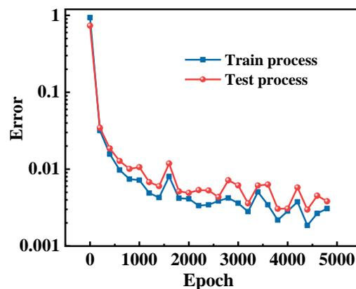
Figure 5. Off-state I–V curve prediction error changes corresponding to different training epochs.
