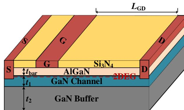
**Figure 1.** Schematic diagram of AlGaIn/GaN HEMT structure.
