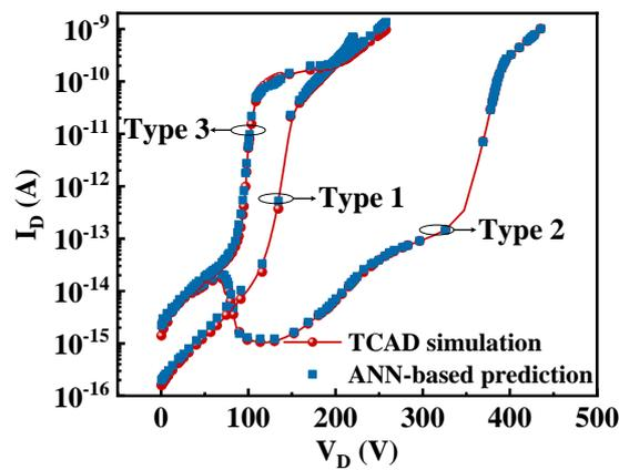
Figure 4. The predicted off-state I–V curve of the ANN-based framework.
