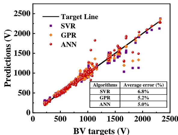
**Figure 8.** The breakdown voltage prediction results from the off-state I–V curve.
