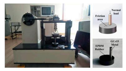
Figure 4. UMT-2 reciprocating test device.
