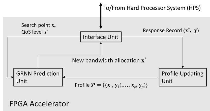
**Figure 2.** The architecture of the proposed FPGA accelerator. It can be separated into three parts: the GRNN prediction unit, the profile updating unit, and the interface unit.
