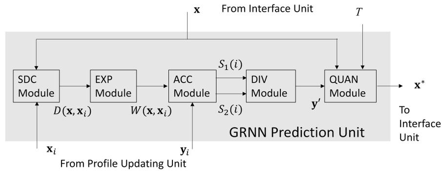
Figure 3. The architecture of the GRNN prediction unit.
