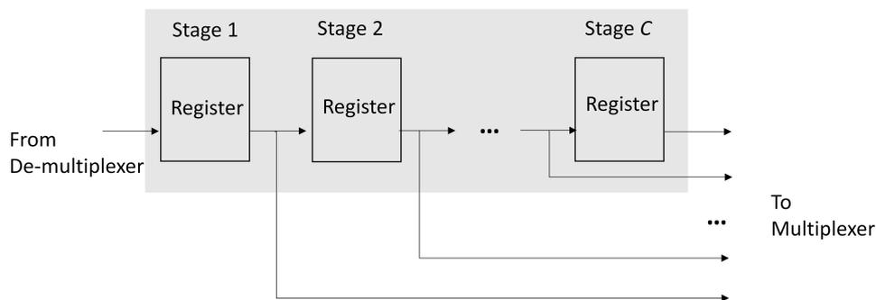
**Figure 8.** The architecture of positive response buffer and negative response buffer. Each buffer is a C-stage shift register supporting SIPO operations.
