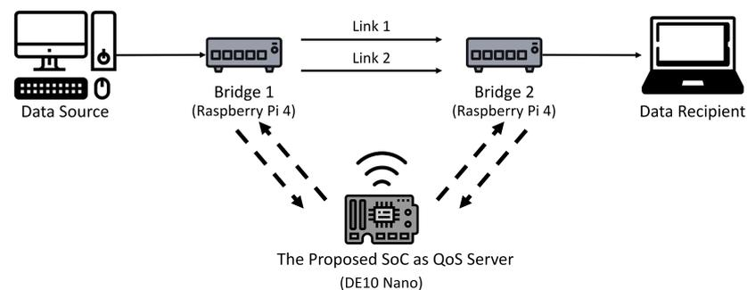
**Figure 11.** The real LAN for the experiments. The proposed SoC is deployed as the QoS server for the LAN.
