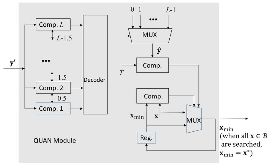
Figure 5. The architecture of the QUAN module.
