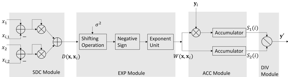
Figure 4. The architectures of the SDC module, EXP module, ACC module and DIV module.
