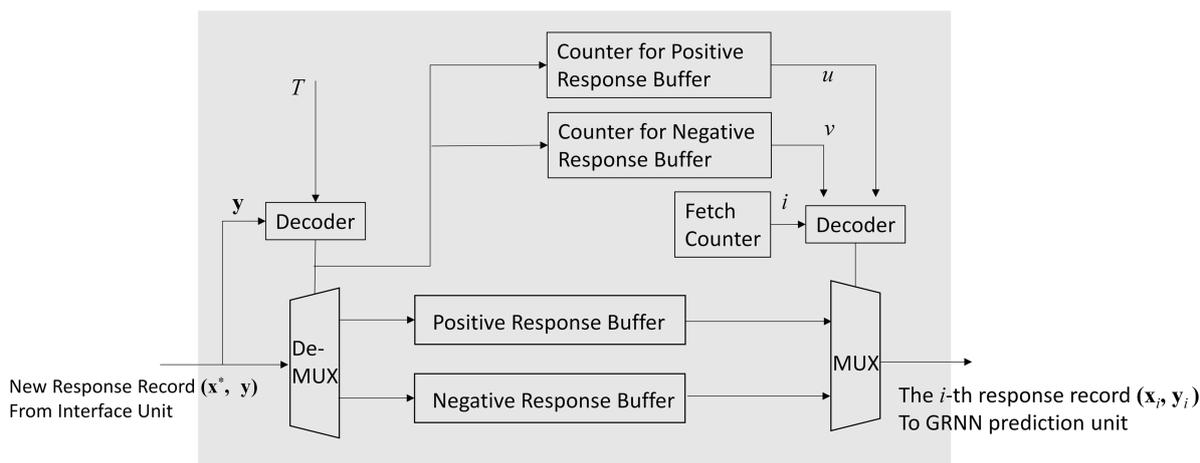
**Figure 7.** The architecture of the profile updating unit. In the architecture, both the positive response buffer and negative response buffer are used for storing response records in  $\mathcal{P}$ .
