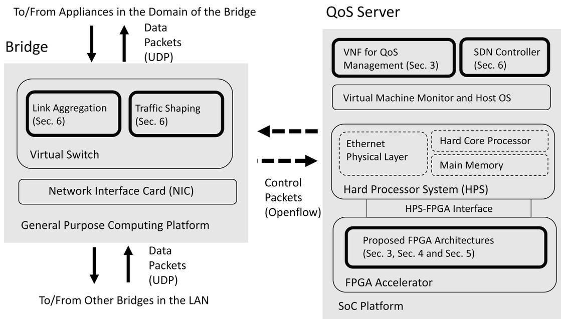
**Figure 1.** The block diagrams of a bridge and a QoS server in the virtual LAN. The bridge is a general purpose computer with a virtual switch. The QoS server is an SoC consisting of FPGA and HPS. In this study, the highlighted blocks are implemented.
