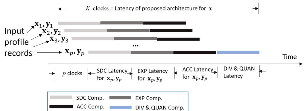
Figure 6. The pipeline operations for the GRNN prediction unit.
