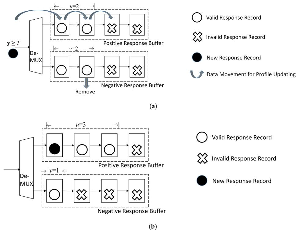
**Figure 10.** A simple example for updating buffers in profile updating unit for  $p = C$ . In this example,  $p = 4, C = 4, u = 2$  and  $v = 2$  before updating. Assume  $y \geq T$  for the new record. The new record is then assigned to positive response buffer. After updating,  $p = 4, u = 3$ , and  $v = 1$ . (a) Before updating; (b) After updating.
