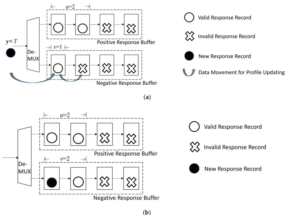
**Figure 9.** A simple example for updating buffers in profile updating unit for  $p < C$ . In this example,  $C = 4$ ,  $p = 3$ ,  $u = 2$ , and  $v = 1$  before updating. Assume  $y < T$  for the new record. The new record is then assigned to negative response buffer. After updating,  $p = 4$ ,  $u = 2$ , and  $v = 2$ . (a) Before updating; (b) After updating.
