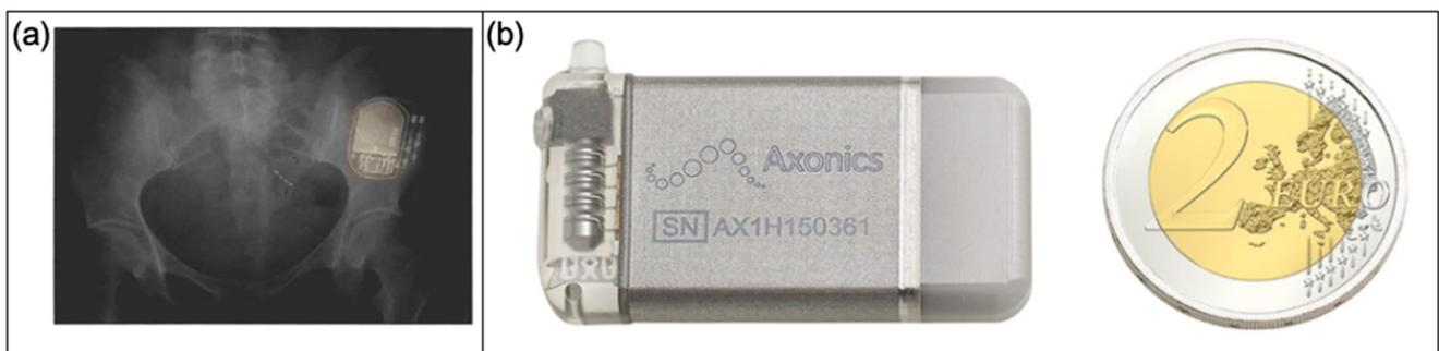
**Figure 3.** Nerve stimulation devices. (a) An anterior–posterior radiograph showing the InterStim device in upper buttock, with a lead electrode in sacral vertebrae (S4) foramen [40]; (b) the Axonics neurostimulator device next to a coin [84]. Copyright 2018, John Wiley and Sons.
