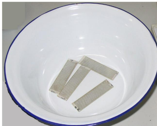
**Figure 9.** IDEs piezoelectric sample (PZT-5).
