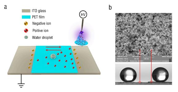
**Figure 4.** Oscillatory motion of droplets on superhydrophobic surface. (**a**) Schematic diagram of the experimental setup. (**b**) Contact angles and surface morphologies of PET film and ITO glass.
