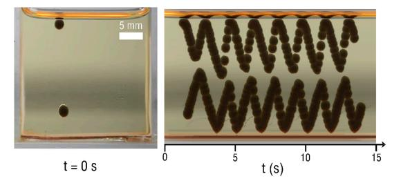
**Figure 3.** Spatial–temporal images of the synchronized oscillatory motion of twin droplets without coalescence at 10 kV.
