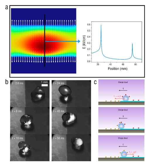
**Figure 6.** (a) Electric field simulation of PET film at voltage of 8 kV. (b) Electrohydrodynamic behavior of water droplet at PET-film boundary. (c) Mechanism for droplet rebound.
