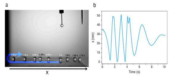
**Figure 5.** (a) High-speed sequential images of the oscillatory motion of a 4  $\mu$ L water droplet under a voltage of 8 kV. (b) Time traces of x coordinate under 8 kV.
