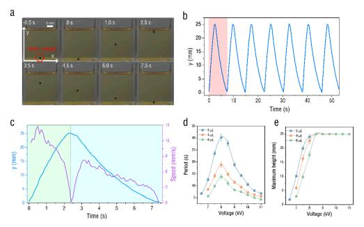
**Figure 2.** Motion of droplet in oil under corona discharge. (**a**) Images of droplet dynamics in the olive oil with the voltage of 10 kV. (**b**) Time traces of y coordinate under 10 kV. (**c**) The displacement and velocity of the droplet versus the time in one cycle. (**d**) Variation of droplet movement period with voltage. (**e**) Change in maximum height of droplet movement with voltage.
