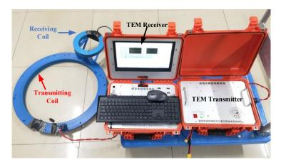
Figure 14. The laboratory simulation comparison test and TEM devices.
